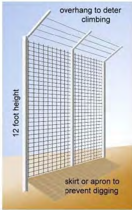
Figure C-1b—Example fence design to deter climbing (e.g., for mountain lions). Source: Vickers and Huber 2012.
