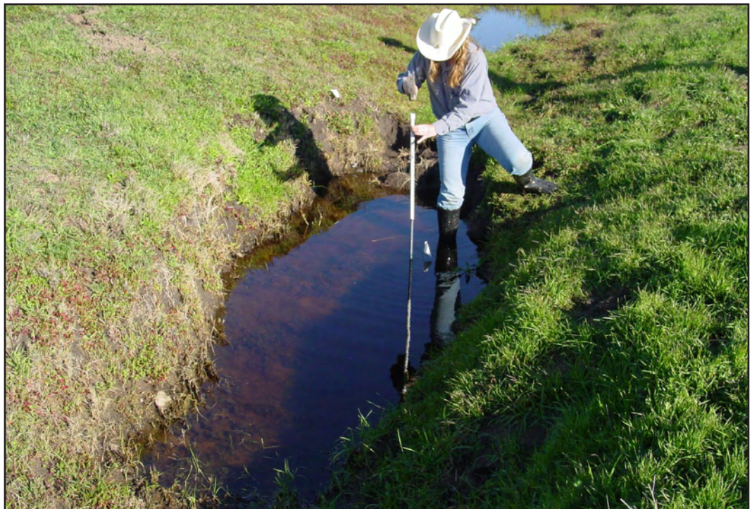
PHOTOGRAPH 16 Vernal Swale vs1, Installing Staff Gauge
