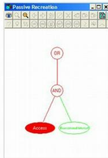
Figure A-3. Knowledge bases for determining passive recreational value. The left panel shows the support for the two conditions of the tested statement: user access ( access ) and resources of recreational interest ( recreational interest ). The right panel shows how the underlying conditions for the user access condition can be obtained by clicking on the access condition, which leads to the results in Figure A-4.
